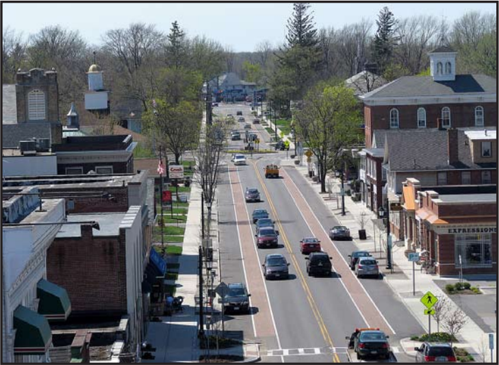
A complete street with on-street parking, wide sidewalks, curb extensions, and well-marked crosswalks
