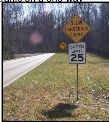
Exhibit 7.10 Example of inappropriate curve speed warning sign
