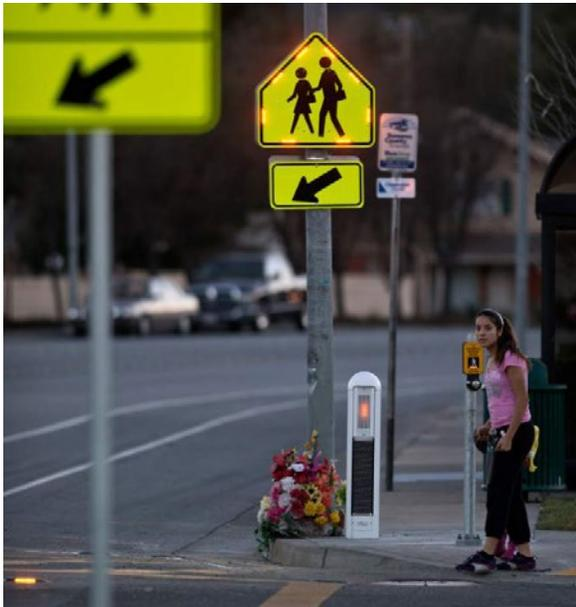
*Pedestrian activated flashing. Photo source: iStock*
