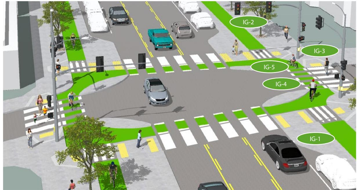
Figure B-13: Partial separated intersection combined with a two-way cycle track and a bike/pedestrian crosswalk. Please note FHWA Separated Bike Lane Planning and Design Guide, as well as emerging best practices for accessibility.
