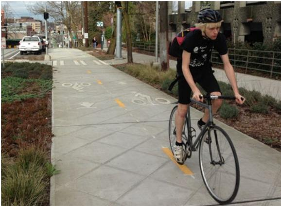
Two-way buffered Cycle Track protected by offset buffers from the roadway. Photo source: Mike Singleton
