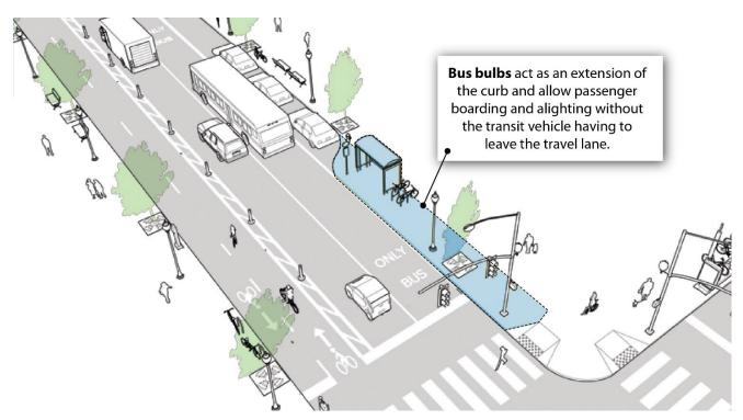
Figure 43. Graphic. Concept demonstrating a bus bulb (adapted from NACTO, 2016).
