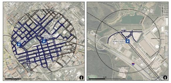
Figure 4. Graphic. Examples of <sup>1</sup>/<sub>2</sub>-mile walksheds for two Dallas area rapid transit rail stations (FTA, 2017).
