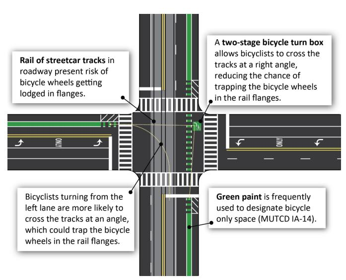
Figure 39. Graphic. Two-stage left turn for bicyclists crossing rail or streetcar tracks. (VHB, 2021).\*
