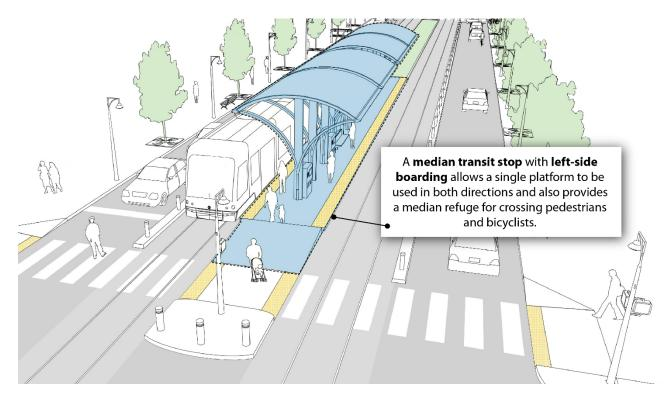
Figure 46. Graphic. Concept demonstrating left side boarding used in both directions (adapted from NACTO, 2016).
