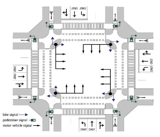
Figure 31. Graphic. Typical signal face locations for motor vehicles, bicyclists, and pedestrians for separated bicycle lanes (MassDOT, 2015).
