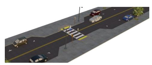
Figure 25. Graphic. Concept demonstrating curb extensions on both sides of crosswalk (VHB, 2018).\*
