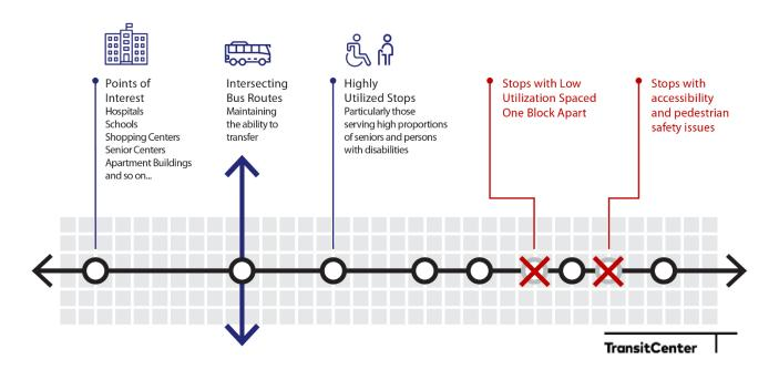
Figure 9. Graphic. Guide to balanced stop spacing (TransitCenter, 2018).
