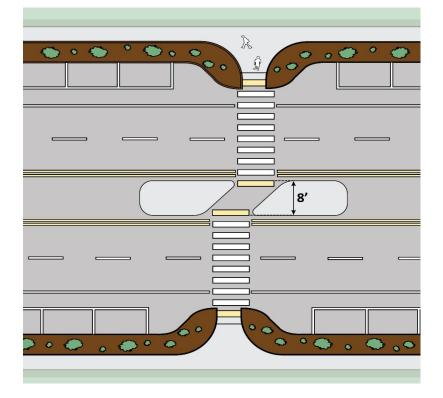
Figure 24. Graphic. Dimension showing pedestrian refuge island crossing width (VHB, 2021).\*
