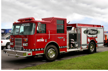
Side-mount pumper, Daytona, FL. Credit: Oshkosh Corporation.
