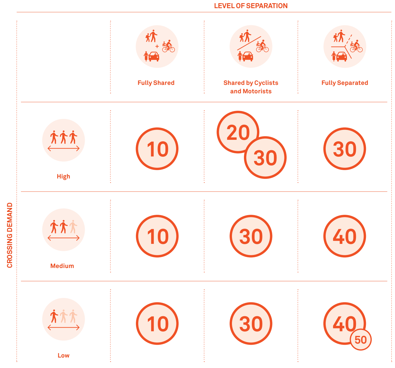
What should my target speed be? Match the Level of Separation and the Crossing Demand of a street to identify the maximum speed for it.
